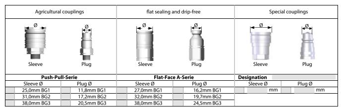
Deviating hydraulic couplings /Include plug with data sheet
