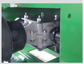
Flat bearing shells for working close to the edge
