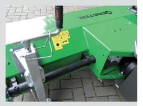
Protected built-in gear for mechanical sweeper
