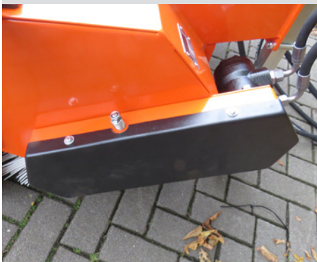
Chain case with maintenance-free chain tensioner
