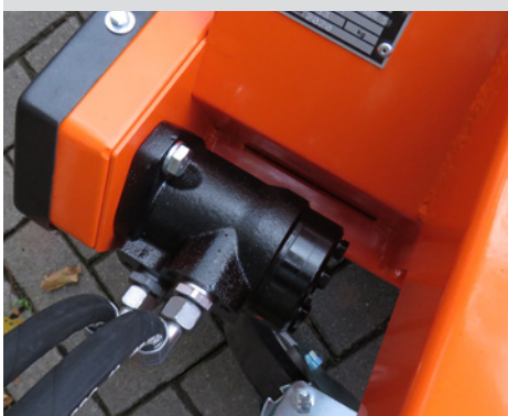
Protected positioned Hydraulic motor
