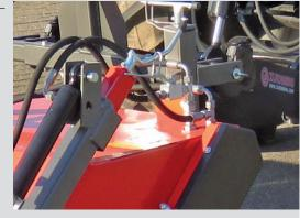
Hydraulically driven side brush with collision safety device and tool-free angle adjustment
