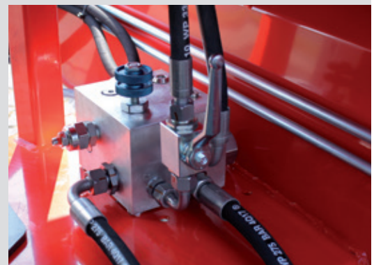
Hydraulic block with all safety functions and free sweeping mode
