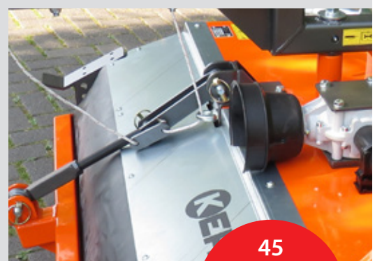
Mechanical Emptying the collection tank (hydraulic optional)
