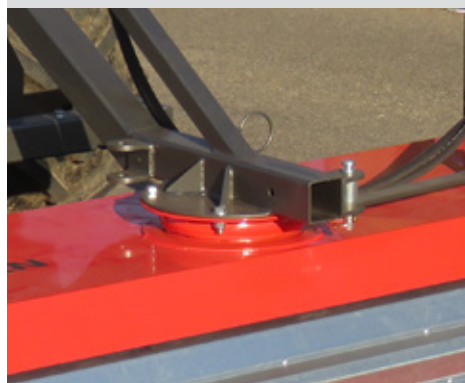
Slewing ring for lateral swivelling (hydraulic adjustment optional)
