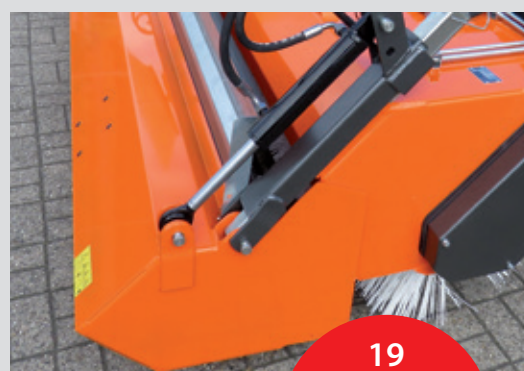
Collecting tank made of steel (option)
