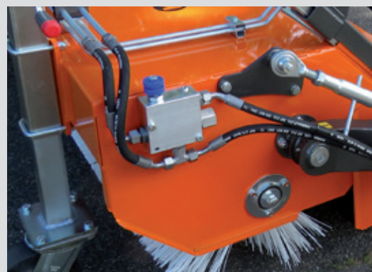
Hydraulics valve for infinitely variable adjustment of the Side brush speed
