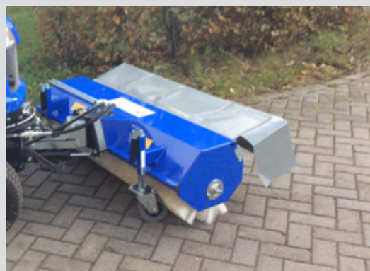
Optional Splash guard for Winter maintenance work
