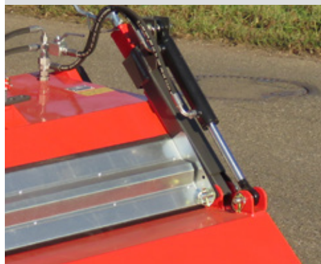
Hydraulic Container emptying
