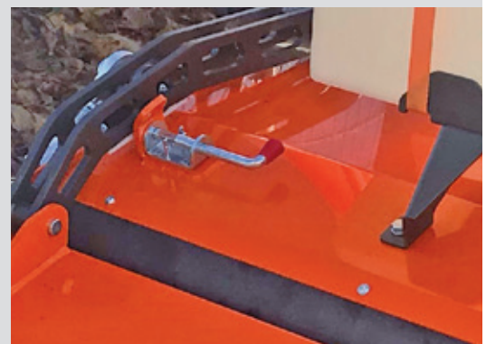
Locking bolt for parking and moving the sweeper
