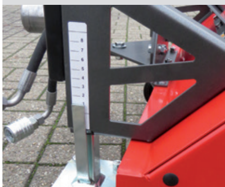
Stepless height adjustment of the sweeper roller
