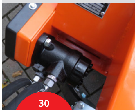
Protected positioned Hydraulic motor
