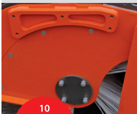
Split side panel for easy change of the sweeper roller
